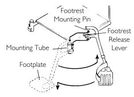
**FIGURE 6.2** Installing/Removing Footrests - 70° Taper
